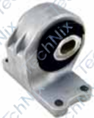
LRD4-T2100 Bracket Assy Mounting (Trans-RR) RNG RVR SPRT V8, LND RVR 3, 4, DISC
